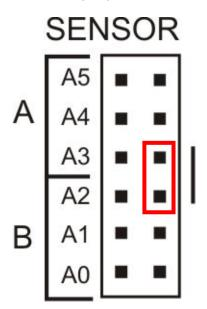
Figure 3. Current sensor jumper block
