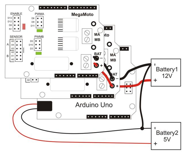
Figure 7. MegaMoto and Arduino connected to different batteries
