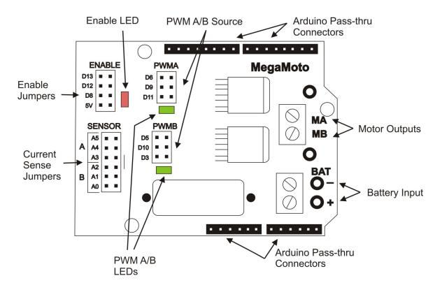
Figure 2. MegaMoto connections and jumpers
