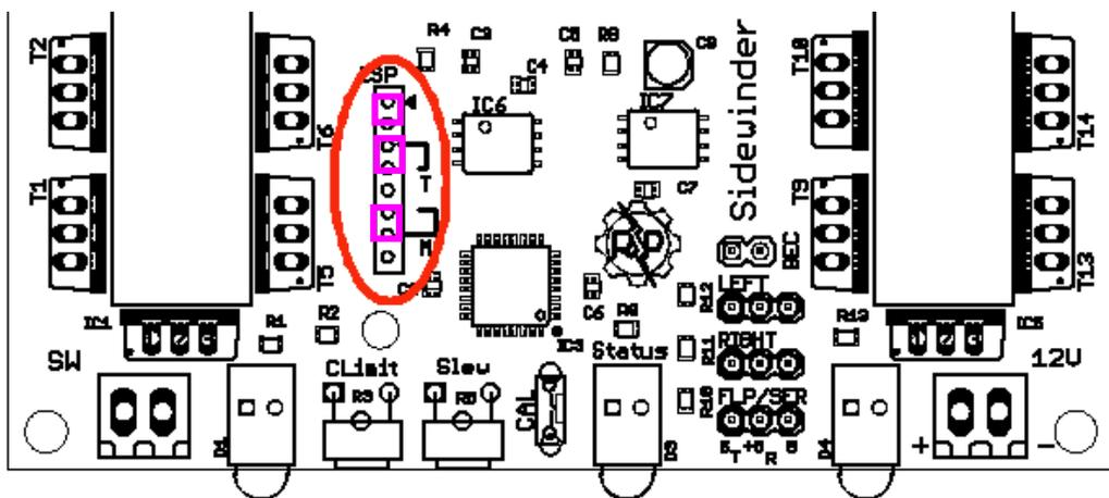
Detection of the operating mode is done at startup. If a mode is selected that requires both Left and Right R/C channels the unit will remain in radio detection mode until signals are received on both Left and Right channels. Note, the behavior of the Sidewinder in Mode 4/5 depends on which R/C channels are connected. The mode
